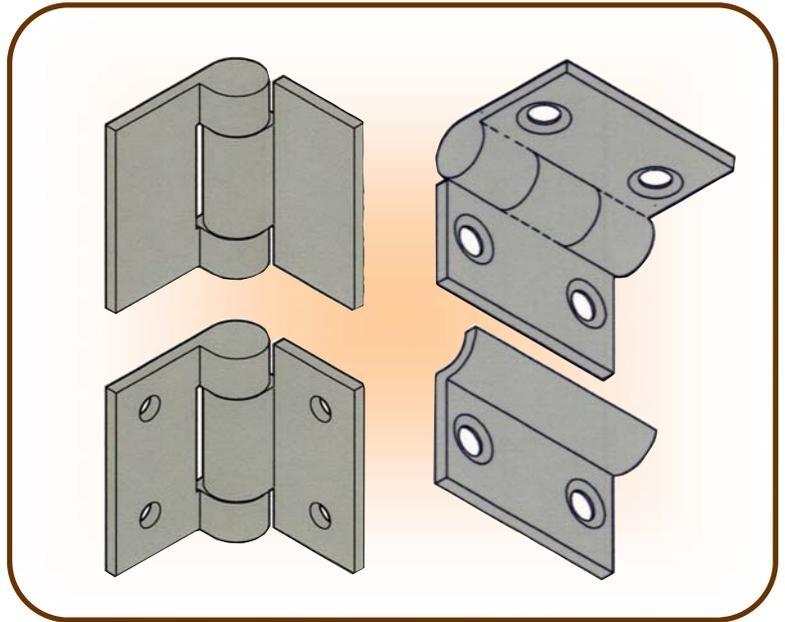
**JCP Specifications:** The JCP 3” full surface weld mount hinge is 3” high x 4” across the leafs, and 1/4” thick cold rolled steel with a USP finish. The hinge has a hardened alloy steel pin that is concealed and non-removable, and a heavy-duty bearings.
